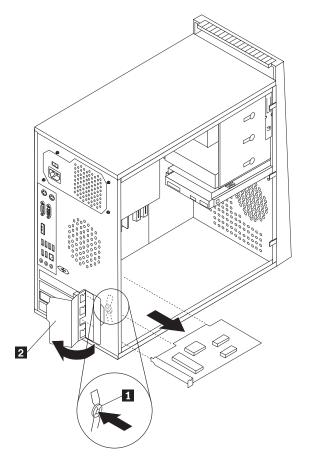
Figure 7. Opening the adapter card latch
